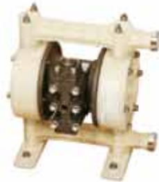
P/N 20013-YPS 1" Double diaphragm pump has polypropylene body construction with Santoprene diaphragm and seals. Rated to 49 GPM maximum capacity with 1" NPTF inlet and outlet, 3/8" NPT air inlet. Operating air pressure from 20 to 100 PSI.
